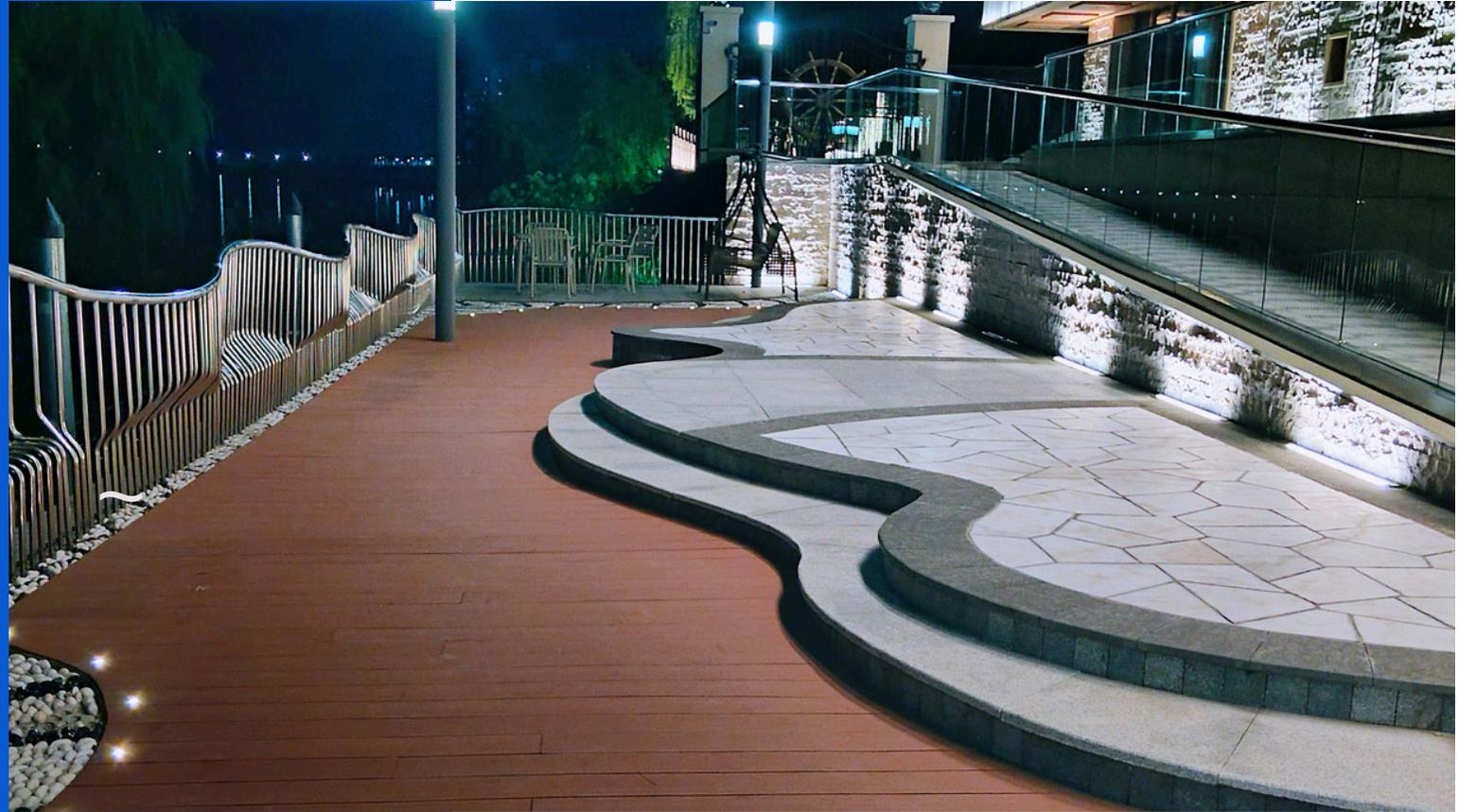
Target Specialties PRE series is the first generation of WPC products made through an extrusion process using wood powder, PE plastic, and additives as raw materials. It offers a wide range of colors. With its high-quality characteristics such as waterproofing, low expansion rate, corrosion resistance, and resistance to moth damage, it is commonly used as an outdoor landscape product in place of real wood and anti-corrosion wood.
